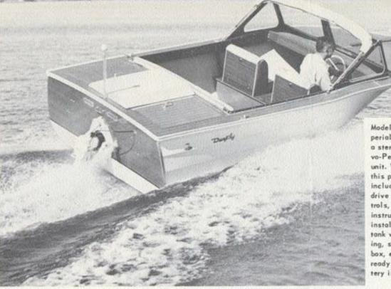
Model 1782 IM Voyager Imperial is also available as a stern drive using the Volvo-Penta Aquanaut 80 h.p. unit. When furnished with this power, the price shown includes the engine and drive unit installed, controls, propeller, standard instruments, permanently installed 18 gallon fuel tank with vent and grounding, sound insulated motor box, electric bilge blower, ready for operation, (Battery is not supplied.)
